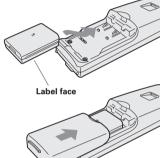
Install the battery pack with the label down.
